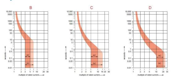
Figure 4 MCB trip characteristic curve
