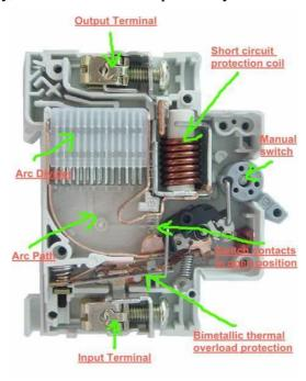
Figure 1 MCB internal structure
