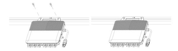
Microinverter can also be installed on the wall. Using the bracket (optional) and fix it on the wall. Then using two pairs of screws and nuts to fix the microinverter on the bracket. Make sure that the label of microinverter should be outside.
