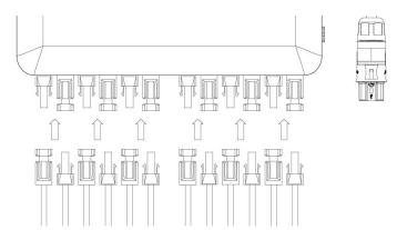
While using PSOL-MS3000L microinverter, each DC input of microinverter can connect two PV modules in series.
