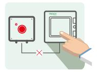
Disconnection of the external AC supply, by whatever means, causes automatic remote operation of the Emergency Rapid Shutdown Switch and solar panel shutdown.
